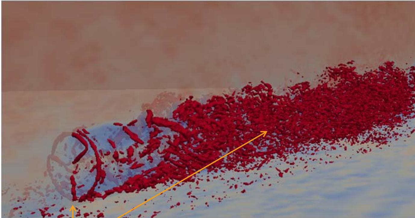
Two NREL 5-MW turbines subjected to neutrally stable low-roughness atmospheric conditions showing the instantaneous streamwise velocity contours with iso-surface of  $Q$  invariant fixed at  $0.0275 \text{ 1/s}$
